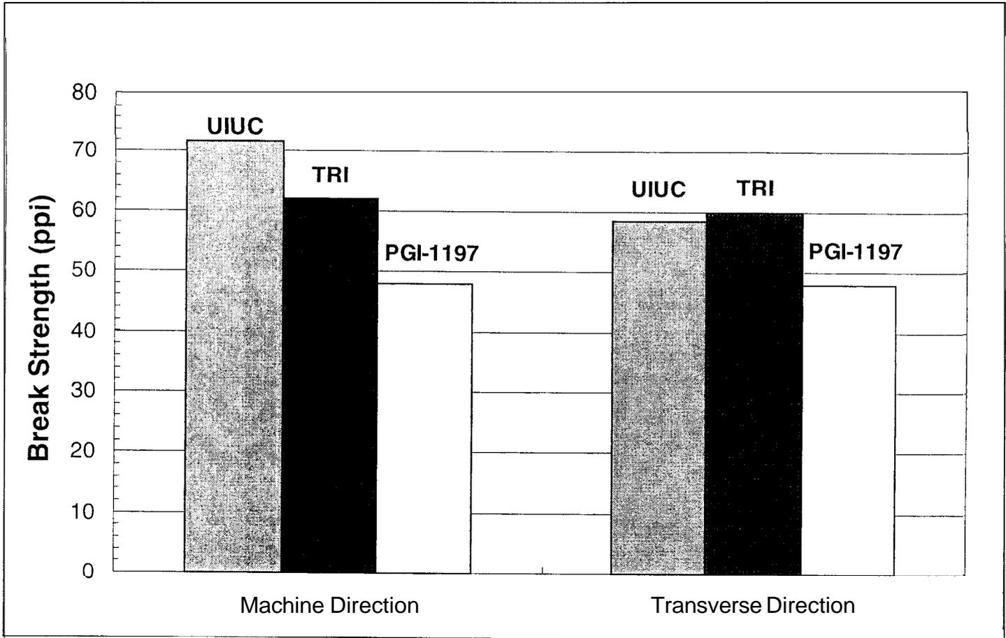
Figure 6: Tensile Break Strengths in the machine and transverse directions compared to the PGI-1197 specification
