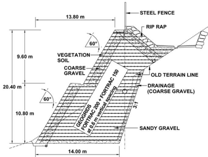
Figure 10. Gondo: typical cross-section of the stone avalanche and rock-fall protective wall
