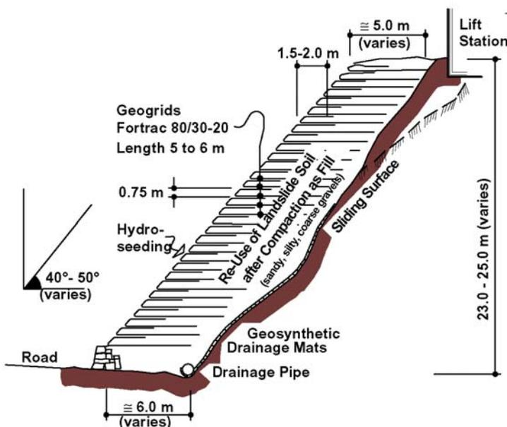
Figure 2. Steinmaderer Wand: typical cross-section of new Fortrac®-geogrid-reinforced slope
