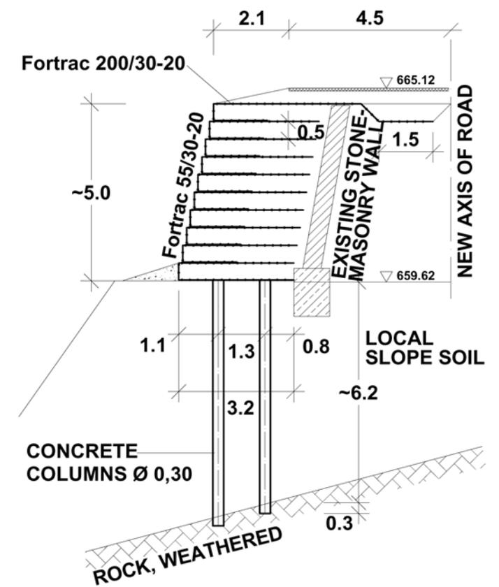
Figure 6. Jugovsko Hanche: typical geotechnical situation and solution with a combined system
