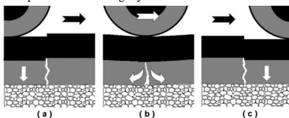
Figure 1- Critical load solicitations in a pavement
