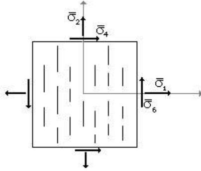
Figure 10 – Unidirectional distribution of slit cracks.
