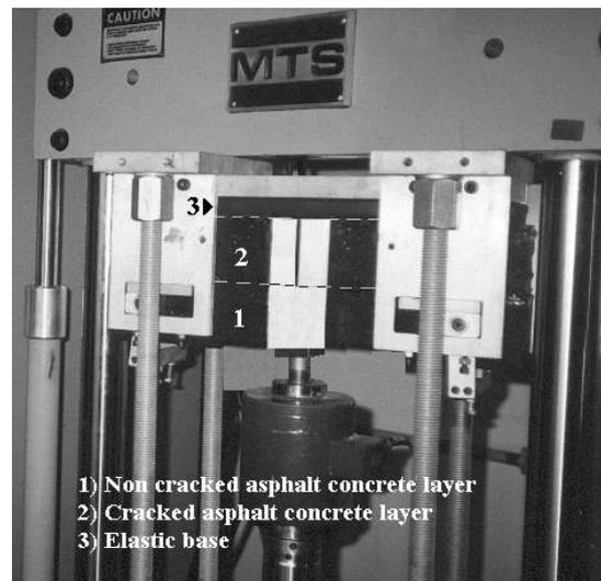
Figure 2 – Fatigue Test with MTS equipment.
