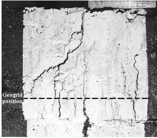
Figure 7 – Beam with geogrid in shearing mode in final stage of the test.
