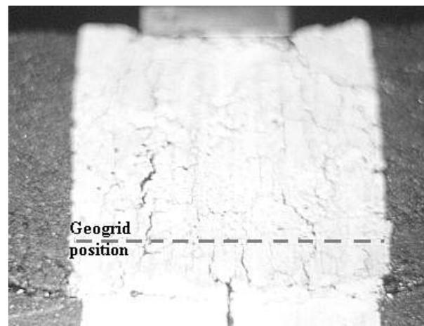
Figure 5 – Beam with geogrid in bending mode
