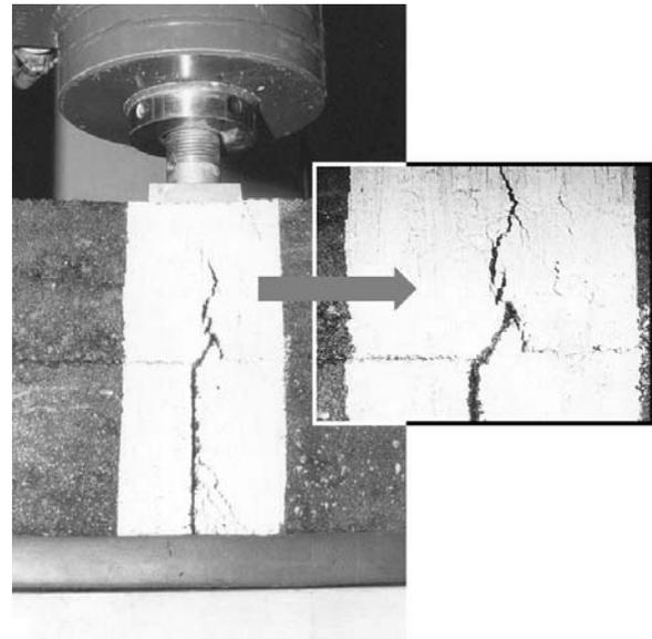
Figure 4 – Crack propagation without geogrid
